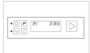
This is the final phase of the program which eliminates the steam created during rinsing, preventing it from escaping into the work environment.
