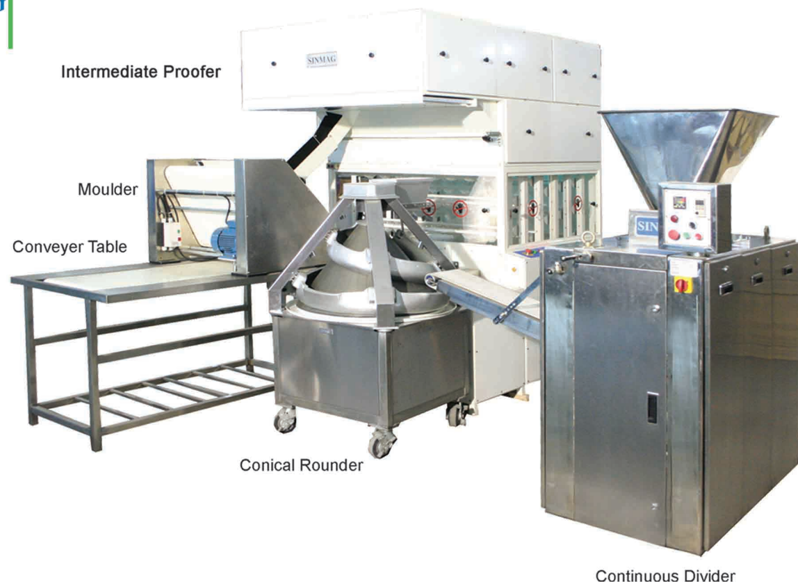
LINE 1) Capacity:1800pcs/Hr;Dough Weight Range:100-300g
